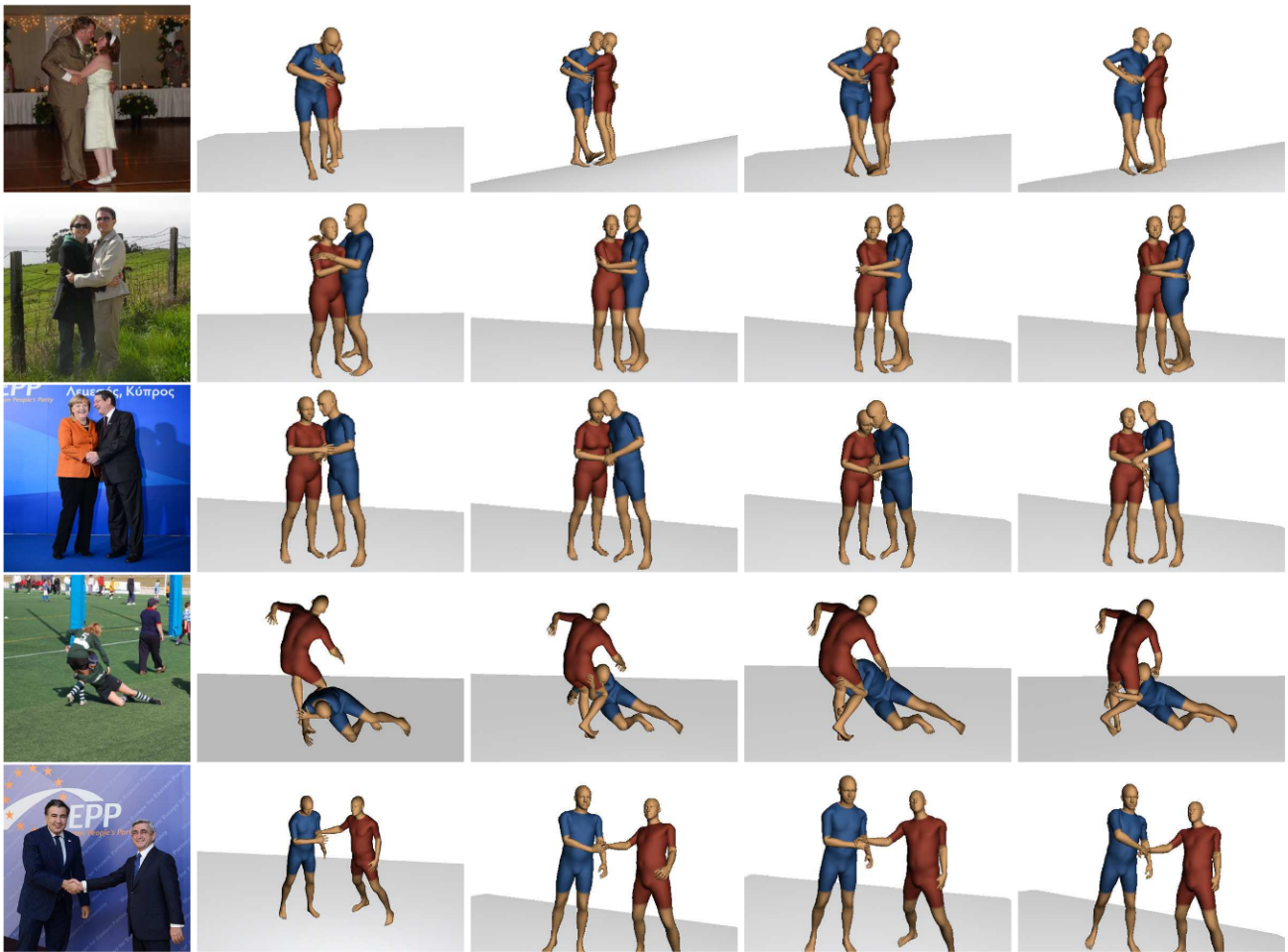
Fig. T1.2.2 3D human pose and shape reconstructions using contact constraints of different granularity. The first column shows the RGB images followed by their reconstructions without contact information (column 2), using contacts based on 37 and 75 regions, respectively (columns 3 & 4), and using facet-based correspondences (column 5). While using facet-based constraints provides the most accurate estimates, reasonable results can be obtained even for coarser (region) assignments.
