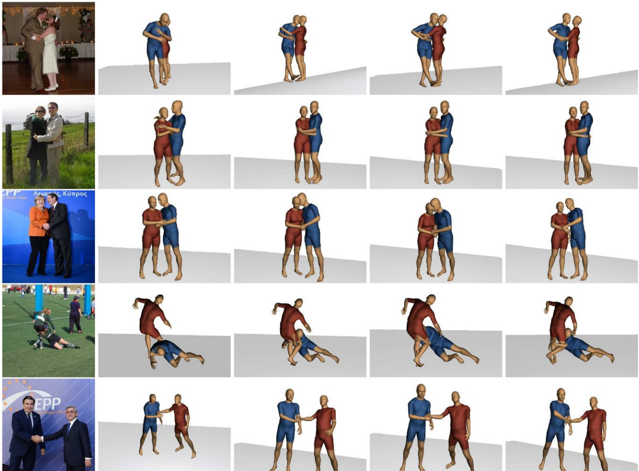
Fig. T1.2.3 3D human pose and shape reconstructions using contact constraints of different granularity. The first column shows the RGB images followed by their reconstructions without contact information (column 2), using contacts based on 37 and 75 regions, respectively (columns 3 & 4), and using facet-based correspondences (column 5). While using facet-based constraints provides the most accurate estimates, reasonable results can be obtained even for coarser (region) assignments.
